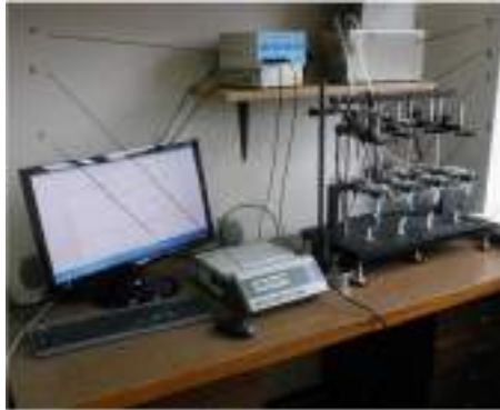
Fig.1. Experimental set-up for the ultrasonic treatment of blood vessel samples (1 – EZ-Bath Tissue/Organ Bath System; 2 – Tissue baths; 3 – Pre-warming System (thermostat); 4 – L-BRAM4 Bridge Amplifier; 5 – Ultrasonic processor VCX130PB; 6 – Piezoelectric transducer and probe; 7 – PC monitor.)
