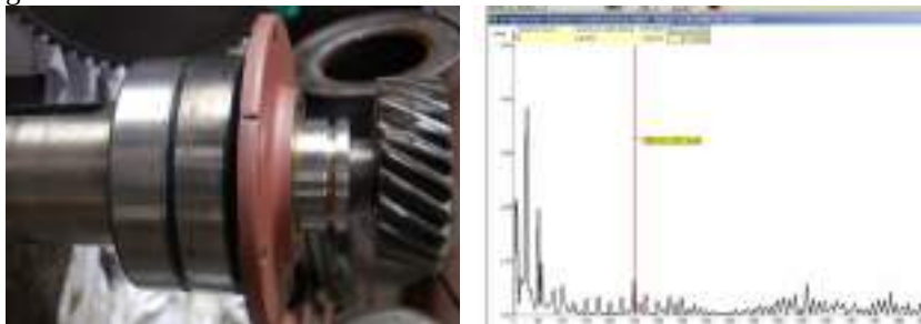
Fig.1. Damaged input shaft with pinion of cooling tower fan gearbox and vibration spectrum when damage was identified. Vibration signal was measured on gearbox case, bearing condition value, RMS value, with unit “g” achieved level 4,98 from 1,25. [JSC “OGP”]
