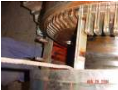
Fig. 1 Driven side view of flexible coupling with heavy damaged plates
