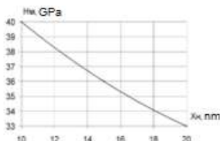
Fig. 3. Dependence of the microhardness of the coating on the grain size
