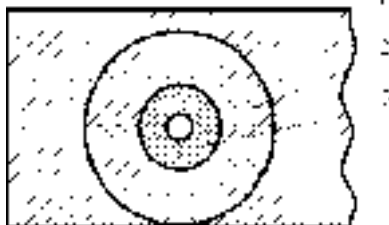
Figure 2 Calculation scheme: 1 - compound; 2 - compound cylinder circled around electronic component; 3 - electronic component
