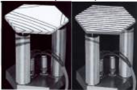
Fig. 4. The mechatronic system with active layered piezoactuators: a- one active layered piezoactuator, b-three active layer ed piezoactuatos
