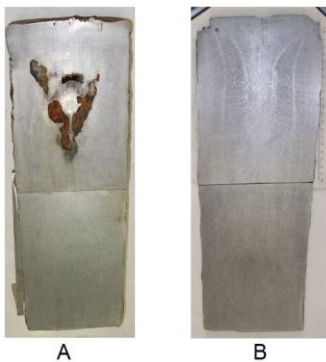
Fig. 3. Macrostructure of experimental ingots: A – without heating and stirring, B – with heating and stirring
