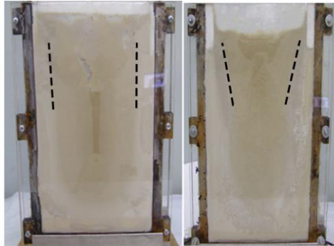
Fig. 2. Effect of heating and stirring on the angle of the crystallization front: A – without heating and stirring, B – with heating and stirring
