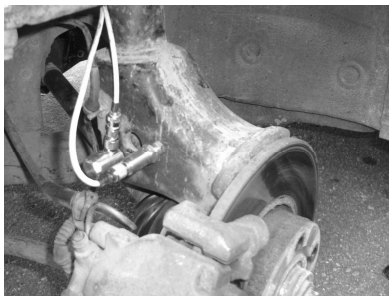
Fig.1. Front wheel support with installed VIB and SPM transducers
